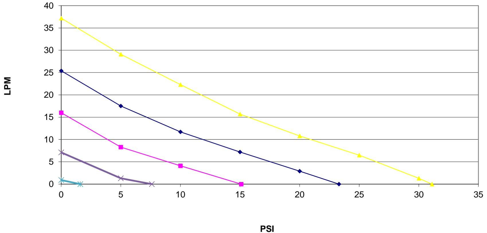
—▲— 0 in Hg    —◆— 5 in Hg    —■— 10 in Hg    —×— 15 in Hg    —\*— 20 in Hg
