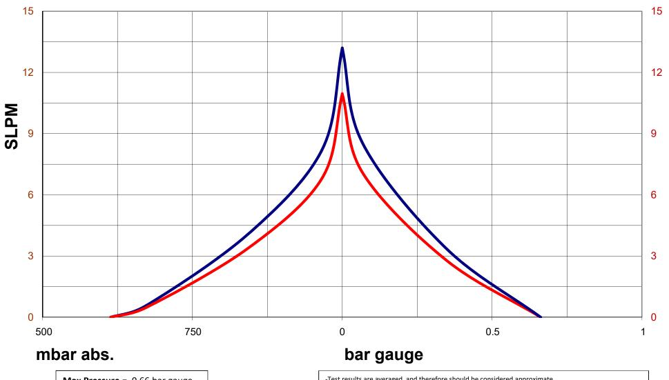
Max Pressure = 0.66 bar gauge Max Vacuum = 614 mbar abs. Max Flow = 13.2 SLPM
