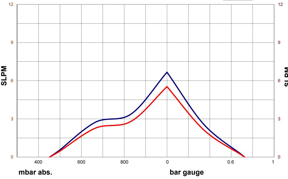
Max Pressure = .7 bar gauge Max Vacuum = 458 mbar abs. Max Flow = 6.7 SLPM
