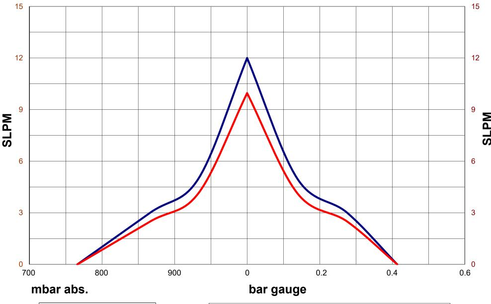
Max Pressure = 0.41 bar gauge Max Vacuum = 766 mbar abs. Max Flow = 12.0 SLPM -Test results are averaged, and therefore should be considered approximate.
