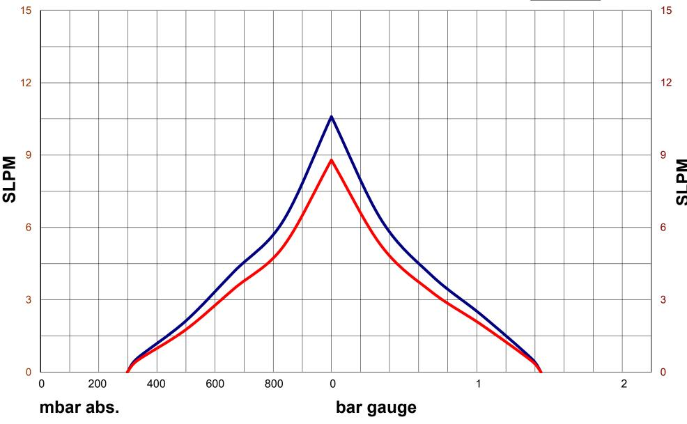
Max Pressure = 1.44 bar gauge Max Vacuum = 302 mbar abs. Max Flow = 10.6 SLPM -Test results are averaged, and therefore should be considered approximate.
