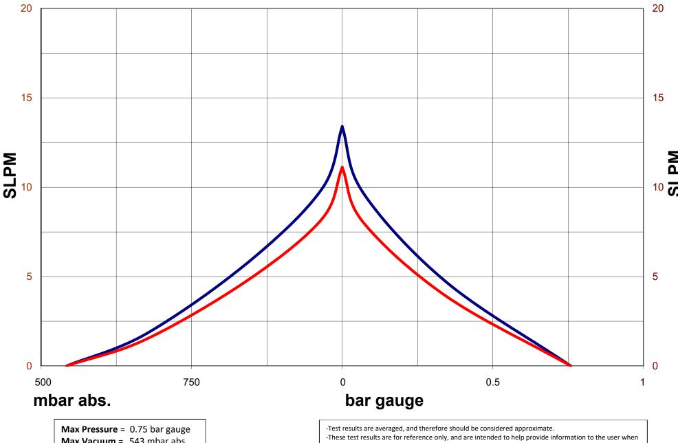
Max Vacuum = 543 mbar abs. Max Flow = 13.4 SLPM
