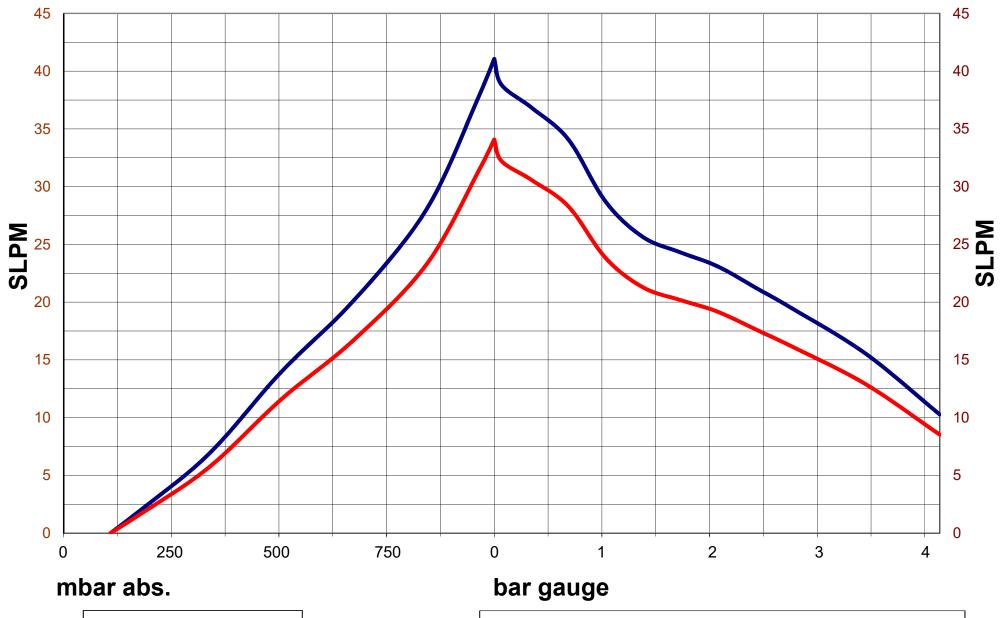
Max Pressure = 4.14 bar gauge Max Vacuum = 109 mbar abs. Max Flow = 41.1 SLPM
