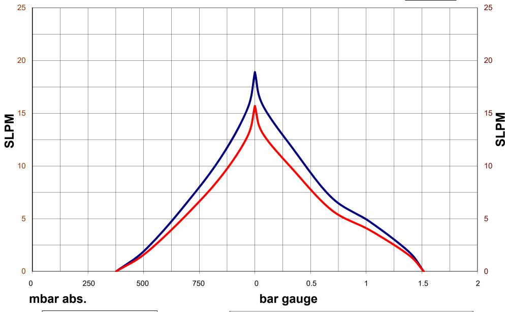
Max Pressure = 1.52 bar gauge Max Vacuum = 377 mbar abs. Max Flow = 18.9 SLPM -Test results are averaged, and therefore should be considered approximate.
