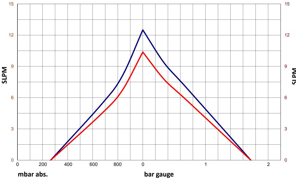
Max Pressure = 1.72 bar gauge Max Vacuum = 268 mbar abs. Max Flow = 12.5 SLPM
