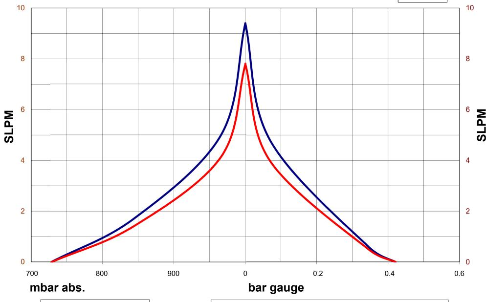
Max Pressure = 0.42 bar gauge Max Vacuum = 729 mbar abs. Max Flow = 9.4 SLPM -Test results are averaged, and therefore should be considered approximate.
