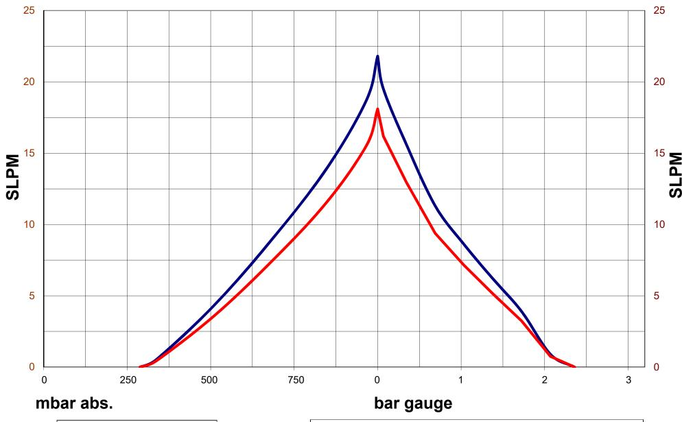
Max Pressure = 2.36 bar gauge Max Vacuum = 288 mbar abs. Max Flow = 21.8 SLPM -Test results are averaged, and therefore should be considered approximate.
