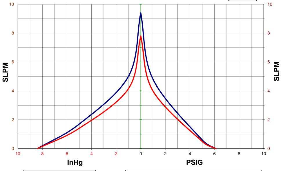
Max Pressure = 6.1 PSIG (0.42 barG) Max Vacuum = 8.4 InHg (284 mBarG) Max Flow = 9.4 SLPM (0.33 SCFM) -Test results are averaged, and therefore should be considered approximate.
