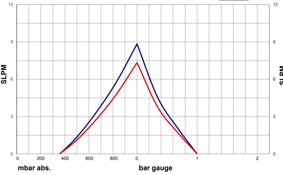
Max Pressure = 1.0 bar gauge Max Vacuum = 363 mbar abs. Max Flow = 8.8 SLPM -Test results are averaged, and therefore should be considered approximate.
