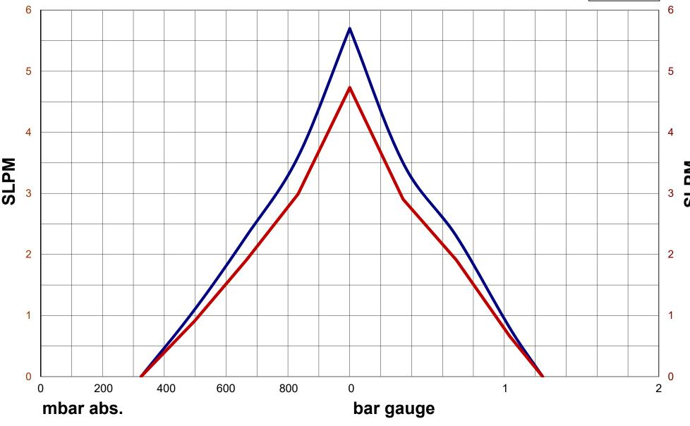
Max Pressure = 1.25 bar gauge Max Vacuum = 329 mbar abs.
