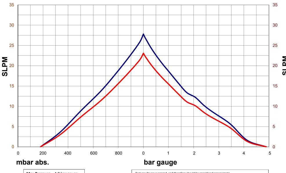
Max Pressure = 4.9 bar gauge Max Vacuum = 180 mbar abs. Max Flow = 27.8 SLPM
