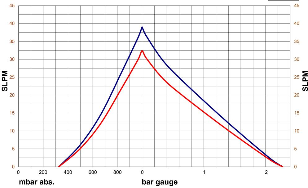
Max Pressure = 2.27 bar gauge Max Vacuum = 329 mbar abs. 39.0 SLPM Max Flow =
